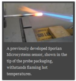
The company's goal is to develop a sensor that improves the ability for active control of combustion instabilities in lean-burning, low-emission aircraft engines. This will enable combustor designs that allow for complete combustion of the fuel while forming fewer pollutants.
